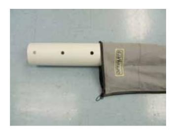
Cut the pipe down to 7 foot 7 inches (91 inches overall). Wrap the sharp ends with some duct tape to prevent the plastic from wearing through the cover. Make sure the tube is clean on the inside before inserting your sail by pushing a damp towel through the pipe using your sprit as a pusher.
